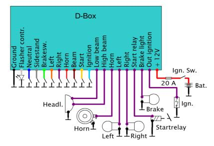
**Push button or switch input for the direction indicators (purple and orange):** You can use these inputs for push buttons or a switch what will connect the input to ground / chassis when pressed. An closed contact will start the indicator. These inputs can also be use for the **2 – Button Mode (Option 6)**.
