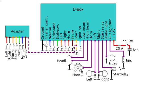
**Push button or switch input for the direction indicators (purple and orange):** You can use these inputs for push buttons or a switch what will connect the input to ground / chassis when pressed. An closed contact will start the indicator. These inputs can also be use for the **2 – Button Mode (Option 6)**.
