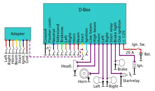
**Push button or switch input for the direction indicators (purple and orange):** You can use these inputs for push buttons or a switch what will connect the input to ground / chassis when pressed. An closed contact will start the indicator. These inputs can also be use for the **2 – Button Mode (Option 6)**.
