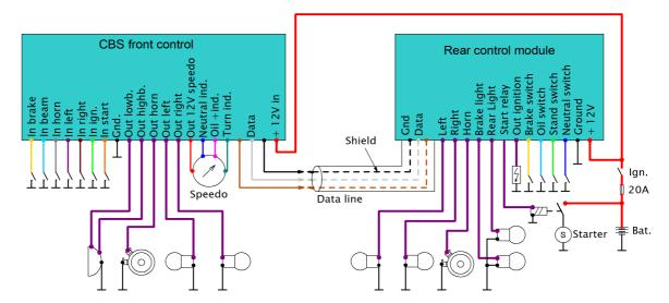
Connect all ground cables to the minus pole of the battery!
