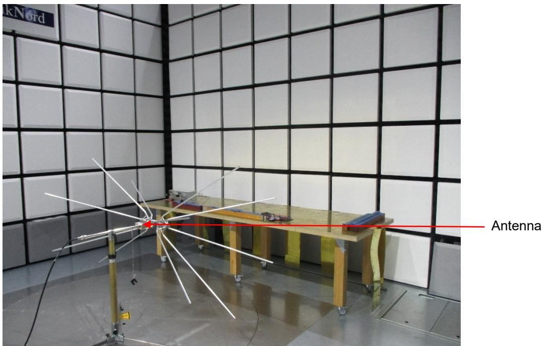
**Fig. 5-8:** Immunity absorber chamber test, 20 MHz – 200 MHz, horizontal
