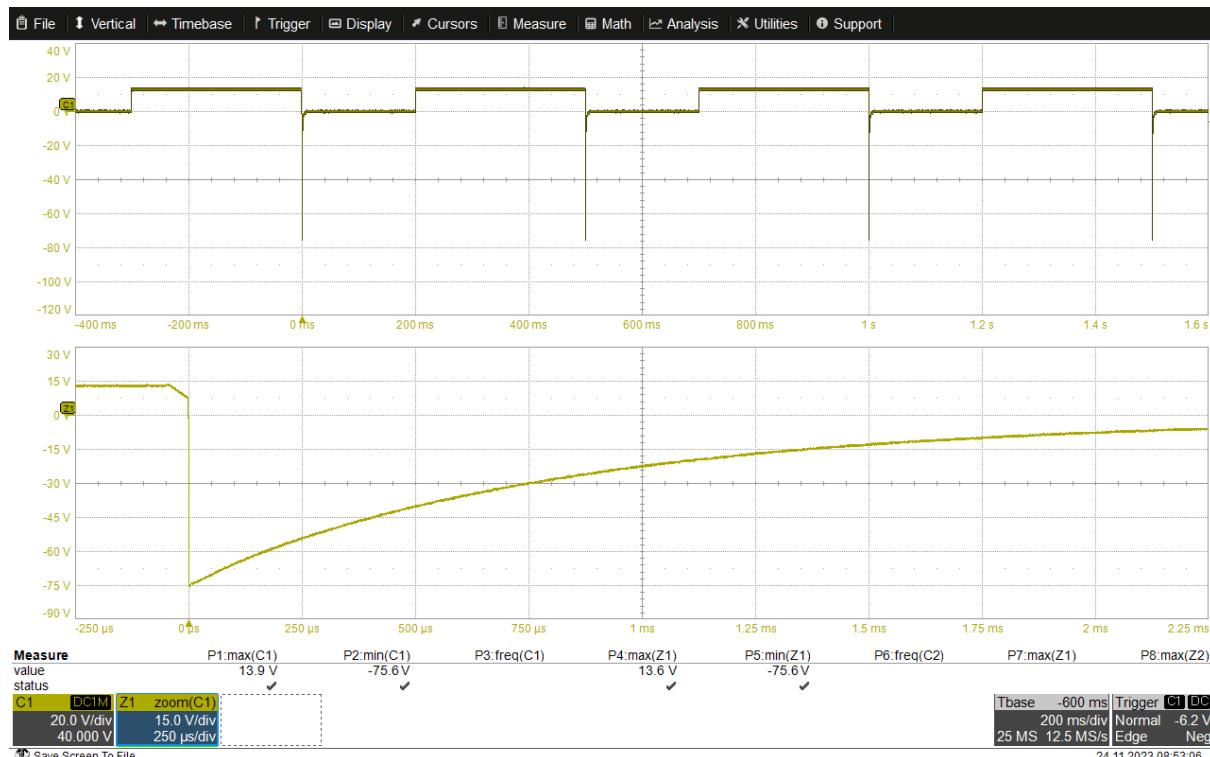
**Diag. 5-11:** Transient immunity test, test pulse 1, t = 200 ms/div
