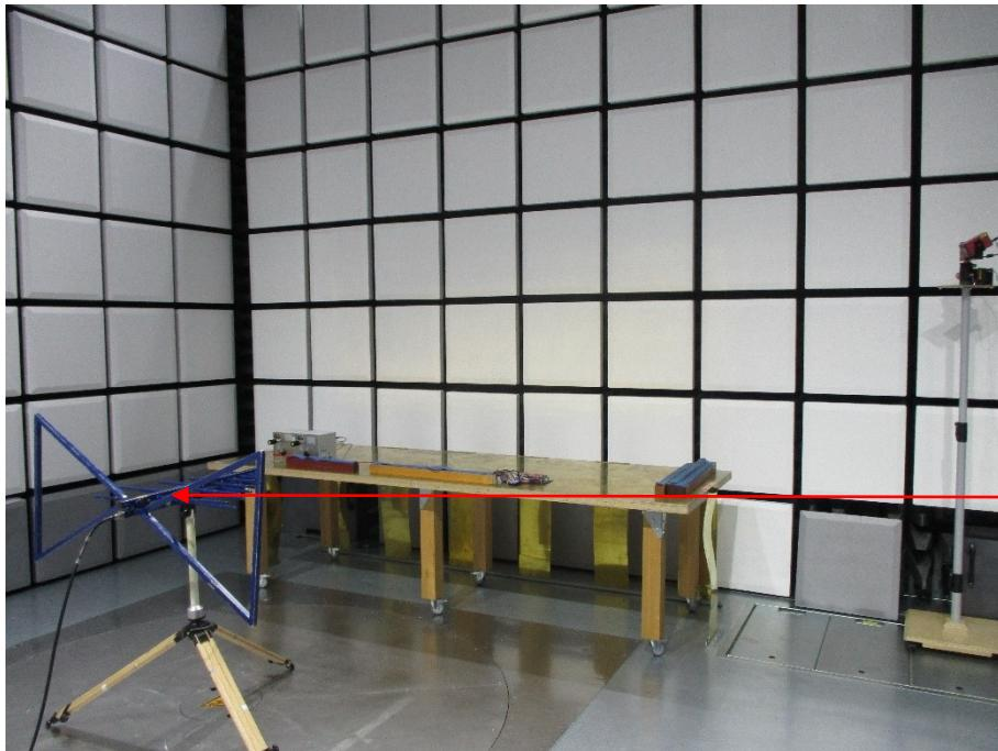
Fig. 5-10: Immunity absorber chamber test, 200 MHz – 1 GHz, horizontal
