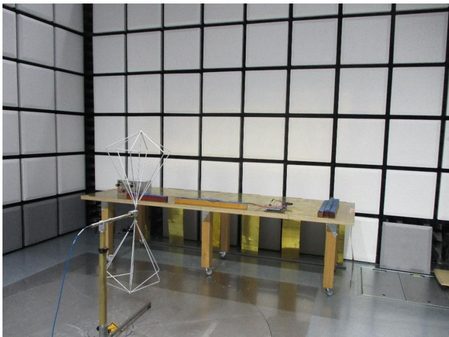
**Fig. 5-2:** Radiated emission broadband, biconical antenna, 30 MHz – 200 MHz, vertical
