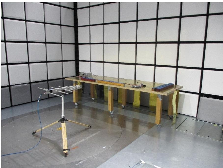
**Fig. 5-3:** Radiated emission broadband, log. -per. antenna, 200 MHz – 1 GHz horizontal
