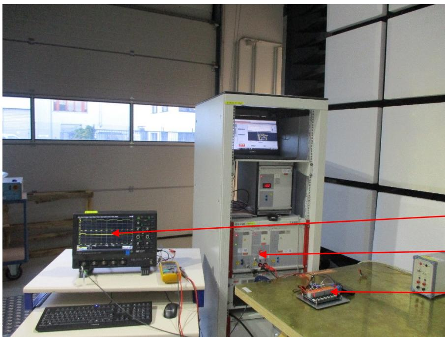
**Fig. 5-14:** Immunity to transient disturbances test setup
