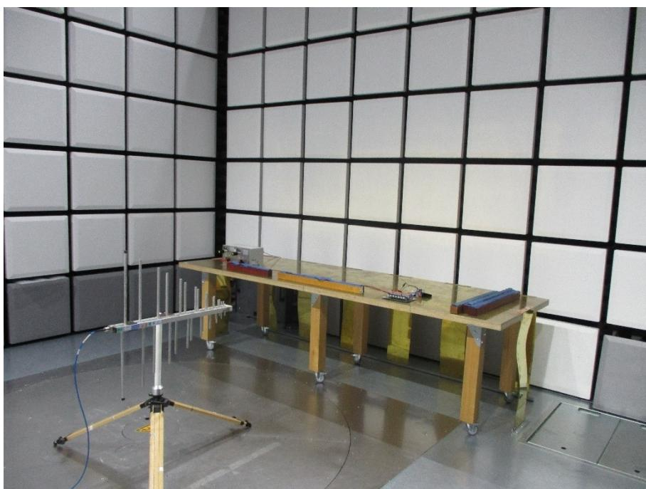
**Fig. 5-4:** Radiated emission broadband, log. -per antenna, 200 MHz – 1 GHz vertical
