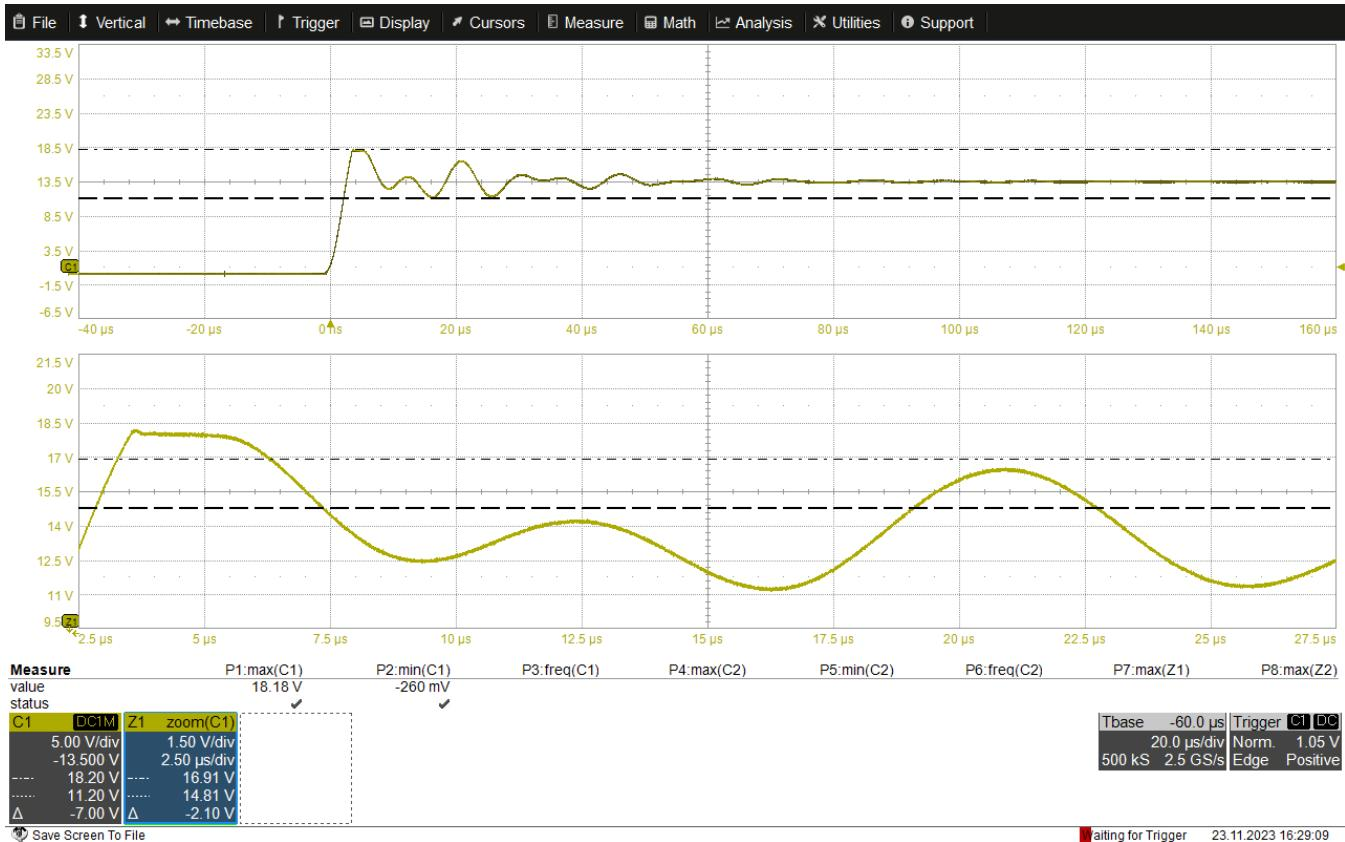
**Diag. 5-7:** Emission of transient conducted disturbances, fast switch on
