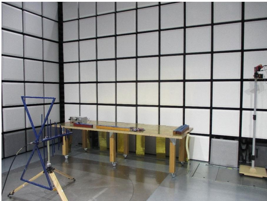
Fig. 5-11: Immunity absorber chamber test, 200 MHz – 1 GHz, vertical
