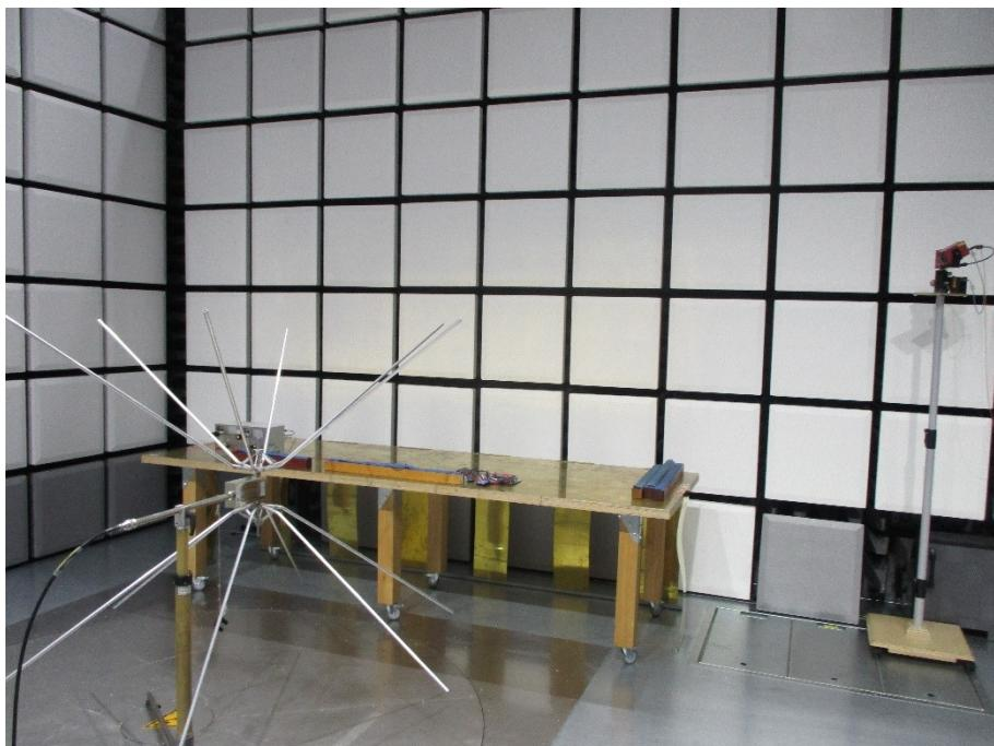
**Fig. 5-9:** Immunity absorber chamber test, 20 MHz – 200 MHz, vertical
