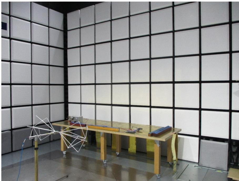
**Fig. 5-1:** Radiated emission broadband, biconical antenna, 30 MHz – 200 MHz, horizontal
